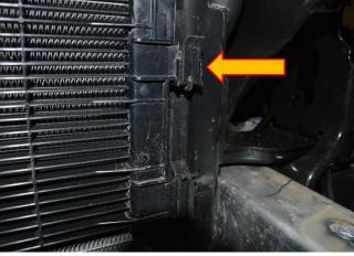
20. Remove the PAS cooler from its brackets BUT DO NOT DISCONNECT FROM ITS HOSES.
