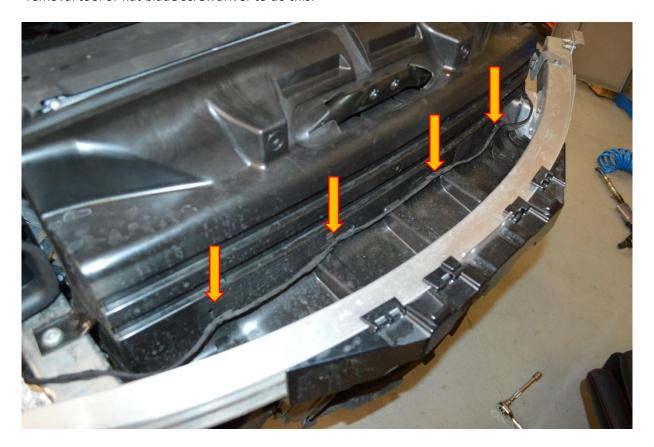
**16.** Undo and remove the two T50 Torx fasteners attaching the metal cross brace, there is one each side of the brace.
