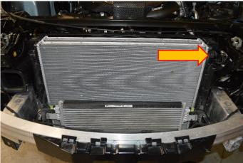
22. The tabs that hold the PAS cooler need to be cut down, use a junior hack saw and make your cut as shown in the picture below. You will need to do this on both sides. There is also a locating pin which needs to snap or be cut off at the top of the radiator.
