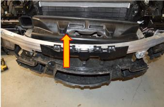
**18**. Remove the radiator top plate, there are two T30 Torx fasteners holding it in place, remove both fasteners and un-clip the top plate.
