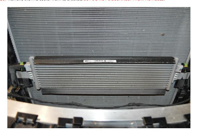
**21**. Remove the lower coupler to drain the charge cooler radiator, then remove the top coupler. Use a flat blade screwdriver to release the spring. You will now be able to lift out the OE charge cooler radiator.
