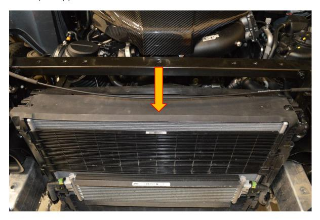
19. Remove upper and lower radiator grills from the OE charge cooler radiator, slide the grill upward while pulling the retaining clip. THESE GRILLS DO NOT GET RE-FITTED.
