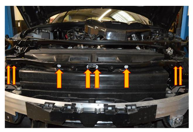
**13**. Use a flat blade screwdriver to prise the retaining clip for the brake ducts. The ducts will pull away to allow access to the lower crash bar fasteners.
